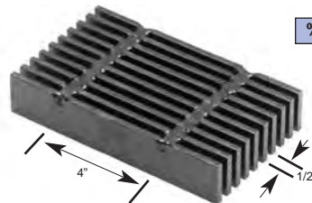
8W4 1/2" Ctr to Ctr of Bearing Bars Cross Rods 4" Center to Center
