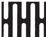
Slot - Side Staggered Round End 1/8" x 1" 43% Open Area
