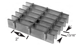
13AP2 13/16" Ctr to Ctr of Bearing Bars Cross Rods 2" Center to Center
