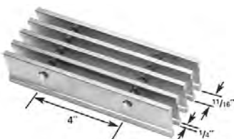
11A14 11/16" Ctr to Ctr of Bearing Bars Cross Rods 4" Center to Center
