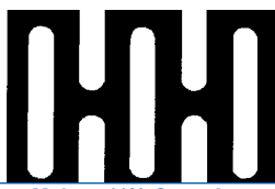
Moire - 41% Open Area 1/8" x 3/4" Round End Slot 1/8" Bars LWS parallel to length of sheet
