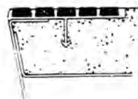
TYPE 231 BF Sure-hold anchor in sloped riser steel pan step.
