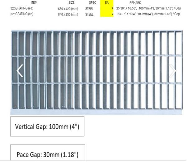
32T Grating means the height is 1 1/4"/ 1.25" and the thickness is 1/4"
