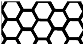
1/4" Honeycomb 1/4" Hex on 9/32" Centers 79% Open Area
