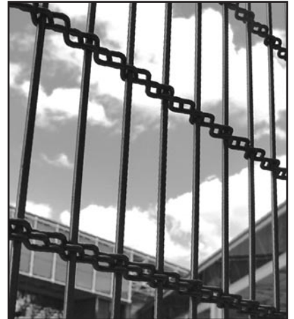
WA-M13Z179 Stainless Steel 304 .120" Gauge % Open Area: 62.9% lbs/sq ft: 1.65 Overall Thickness: .304" Aspect Ratio: 8.16:1
