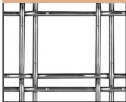
WA-M2227 Carbon Steel & SS304 .162" Gauge % Open Area: 75% lbs/sq ft: 1.40 Overall Thickness: .324" Aspect Ratio: 1:1
