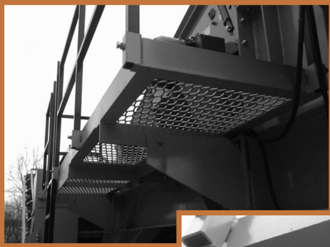
Expanded Metal utilized on Rock Crushing Machinery
