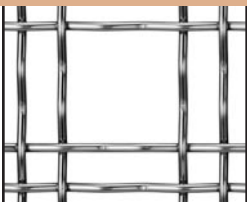
WA-M228 Carbon Steel .162" Gauge % Open Area: 77.2% lbs/sq ft: 1.33 Overall Thickness: .324" Aspect Ratio: 1:1
