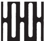
Slot - Side Staggered Round End 1/8" x 1" 43% Open Area
