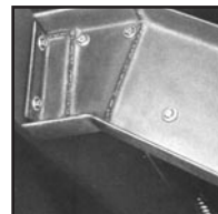
Stringer bolted solidly to top support
