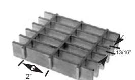
13AP2 13/16" Ctr to Ctr of Bearing Bars Cross Rods 2" Center to Center
