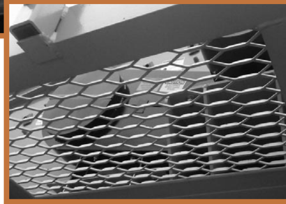
Expanded Metal utilized on Rock Crushing Machinery
