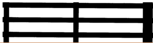
Airline - 68% Open Area 1/4" x 1-1/2" Rectangular Slots Straight row parallel to width 3/32" bar every 3rd bar 3/16" lengthwise. LWS parallel to width of sheet
